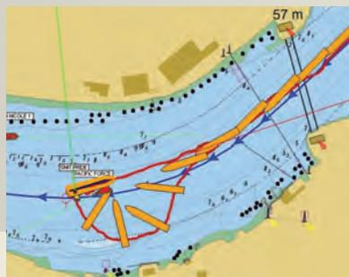
On December 14th, 2012, at 22:00, during an otherwise typical pilotage assignment on the Fraser River, the bulk carrier *Star Grip* had an engine failure with other vessels and marine infrastructure in close proximity. This screenshot from Pilot Randy Smigel's portable pilot unit shows how he immediately used the vessel's anchor to slow it down as he conducted a 360 degrees turnaround to safely bring the vessel to a halt. Just another day on the job.
