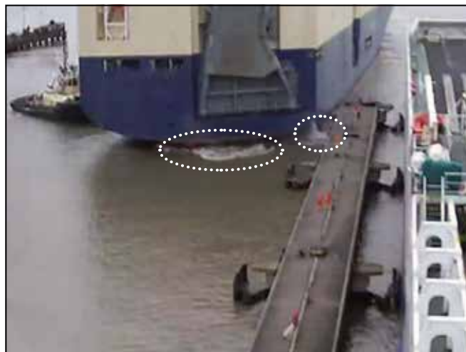
Figure 4: Vessel engine and rudder used after collision and damage to tank causing leak
