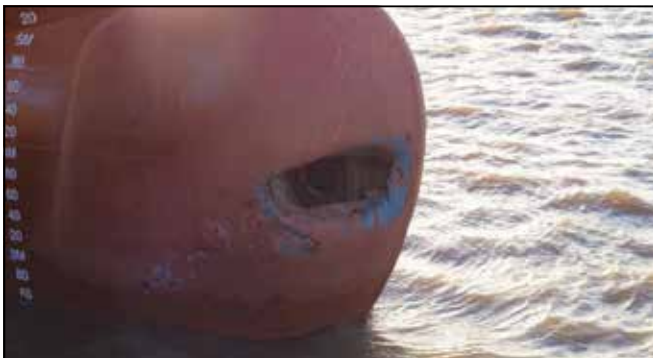
Figure 1: Bulbous bow damage caused by contact with the quay
